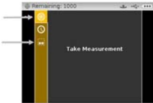
Fig.11 Moving from measurement mode to groups mode.
